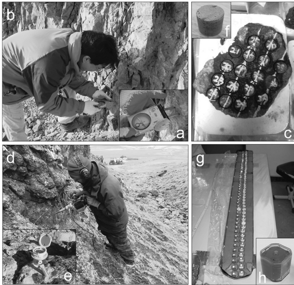
Fig. 3 Photos showing sample collection methods. (a) tripod compass; (b) hand sampling from outcrop; (c) plaster method; (d) drill sampling from outcrop; (e) orientator; (f) rock specimen; (g) cube sampling from sediment core; (h) cube specimen.
